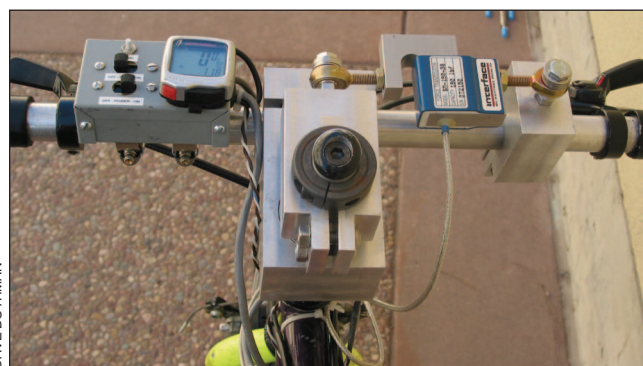
Figure 16. The handlebar of the instrumented UCSB bicycle. Steer torque is measured using a strain gauge on the right. The box on the left contains a display for speed and switches for data logging.
