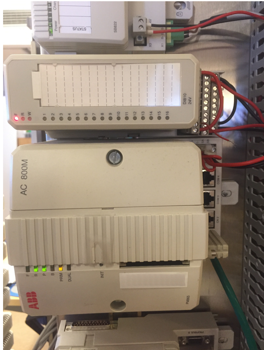
Figure 25: We have performed test runs of Bloqqi programs on AC 800M controllers by ABB. The controller was not connected to any physical process, but we were able to see the values computed by the Bloqqi program by using the Control-Builder software.
