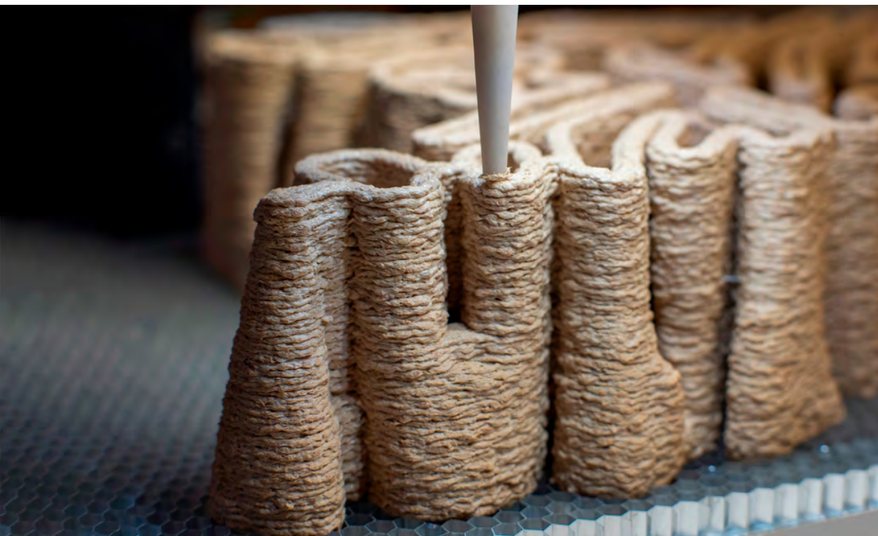
Fig. 7. 3d printing with living pulp.
