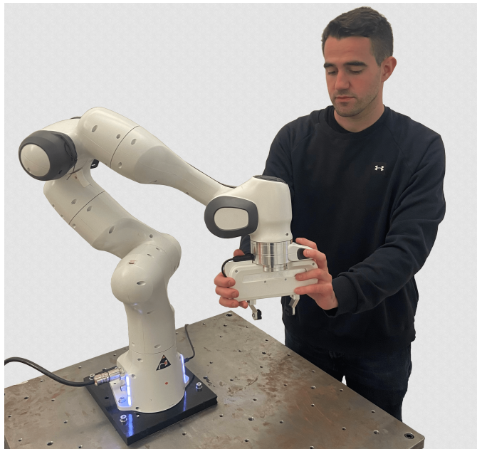
Fig. 1. A human–robot collaborative scenario where an operator was guiding a Franka Emika Panda robot mounted on a table.
