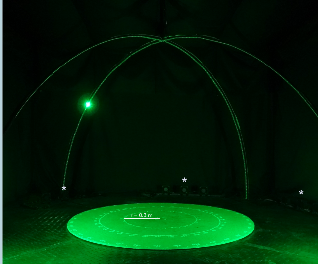
Figure B1: Simulating sun and wind. Behavioural setup consisting of two metal arches lined with green LEDs (520 nm, each simulating a sun), wind generators (asterisks), and a circular, wooden arena with its perimeter labelled from 0-355°. From Paper III.
