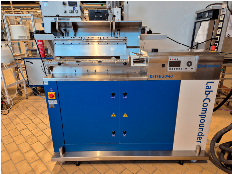
Figure 13. The laboratory twin-screw extruder with co-rotating intermeshing screws used in this doctoral thesis (TwinLab-F 20/40, Brabender GmbH & Co.KG, Duisburg, Germany).
