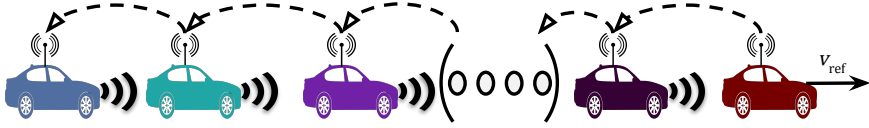
Figure 3.5 A vehicle formation implementing a serial consensus controller. Each vehicle measures the relative distance and velocity to the predecinging vehicle and signals the perceived relative distance to its follower.
