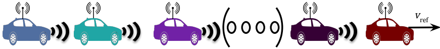
Figure 3.1 Vehicle formation where each car uses onboard sensors to coordinate with its predecessor.
