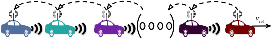
Figure 1.4 Extended vehicle platoon architecture: each vehicle measures the distance to its immediate predecessor and message-passes this measurement to its follower.
