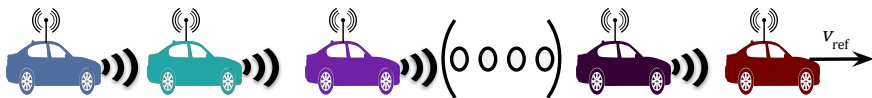
Figure 1.1 A vehicle platoon where each vehicle only measures distances to its nearest predecessor neighbor.
