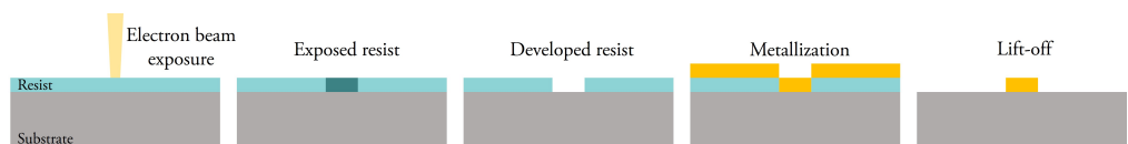
Figure 4.9: A cross-sectional view of EBL process.
