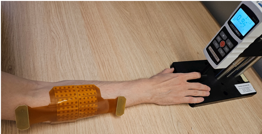
Fig. 1. The placement of the high-density electrode grids on the dorsal side of the proximal half of the right forearm, and the index finger position pushing upwards against the force gauge.
