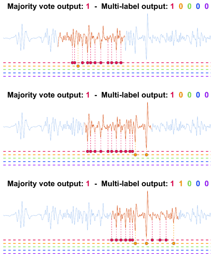
Figure 3. The moving window classification procedure is illustrated on the same EMG channel (light blue lines) overlapped with the 250 ms moving window (red line), for three different segments with a 100 ms stride. The horizontal dashed lines represent the five classes. The coloured dots denote the identified peaks on the line of their assigned class. Using single label majority voting, all cases in this example were classified as thumb extension (red). In the multi-label case, with a minimum threshold of 3 peaks, the last window was classified as both thumb (red) and index (orange) extension.
