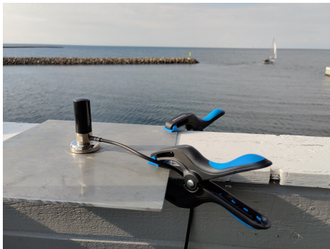
Figure 1: Base station antenna (Rx) with a clear view on the sea, and a sailing boat in the background which acts as UE (Tx).
