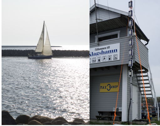
Figure 2: Photographs of the sailboat (Tx) and the vertical array (Rx) ashore.
