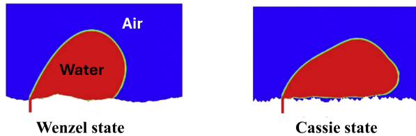
Figure 2.6: Typical Cassie 1 and Wenzel 2 states of a droplet on rough GDL surfaces. Figures are adapted from Bao et al. (International Journal of Hydrogen Energy, 2020) [128], with permission from Elsevier.
