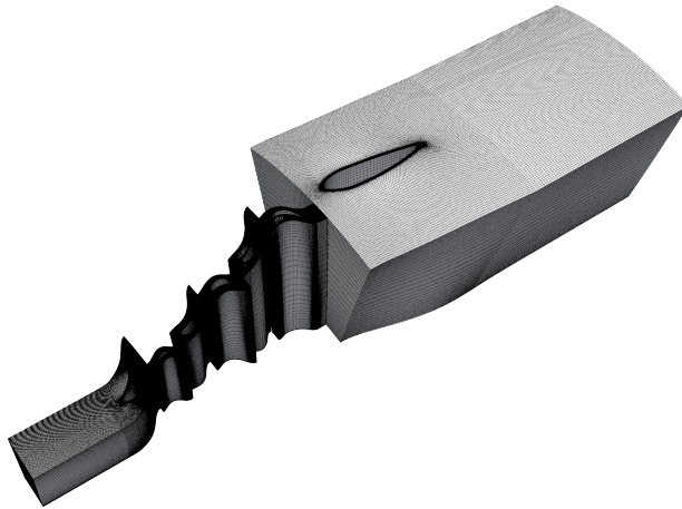
Figure 4.6: Structured O, C, and H-type mesh topology for the computational domain of the multistage axial gas turbine in Paper IV, showing one channel passage; the final full-annual 3D mesh contained approximately 66.1 million nodes and 62.5 million elements.
