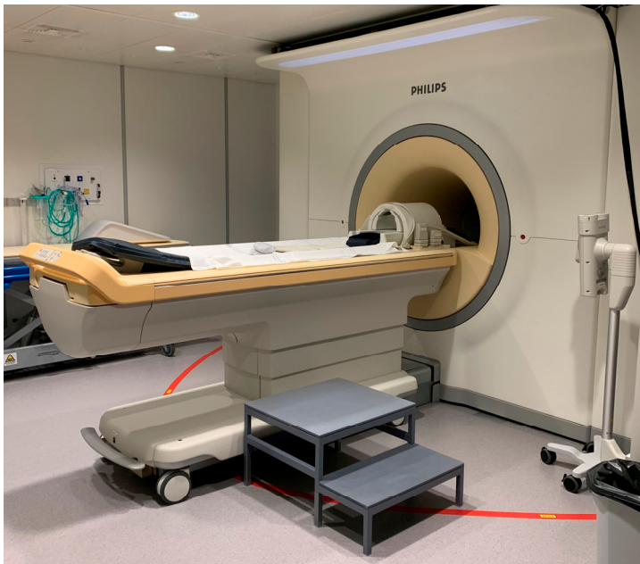
Figure 8. The 7T MR scanner (Achieva 7T; Philips) used in study II-III of this thesis. Image credit: Simon Götstrand.
