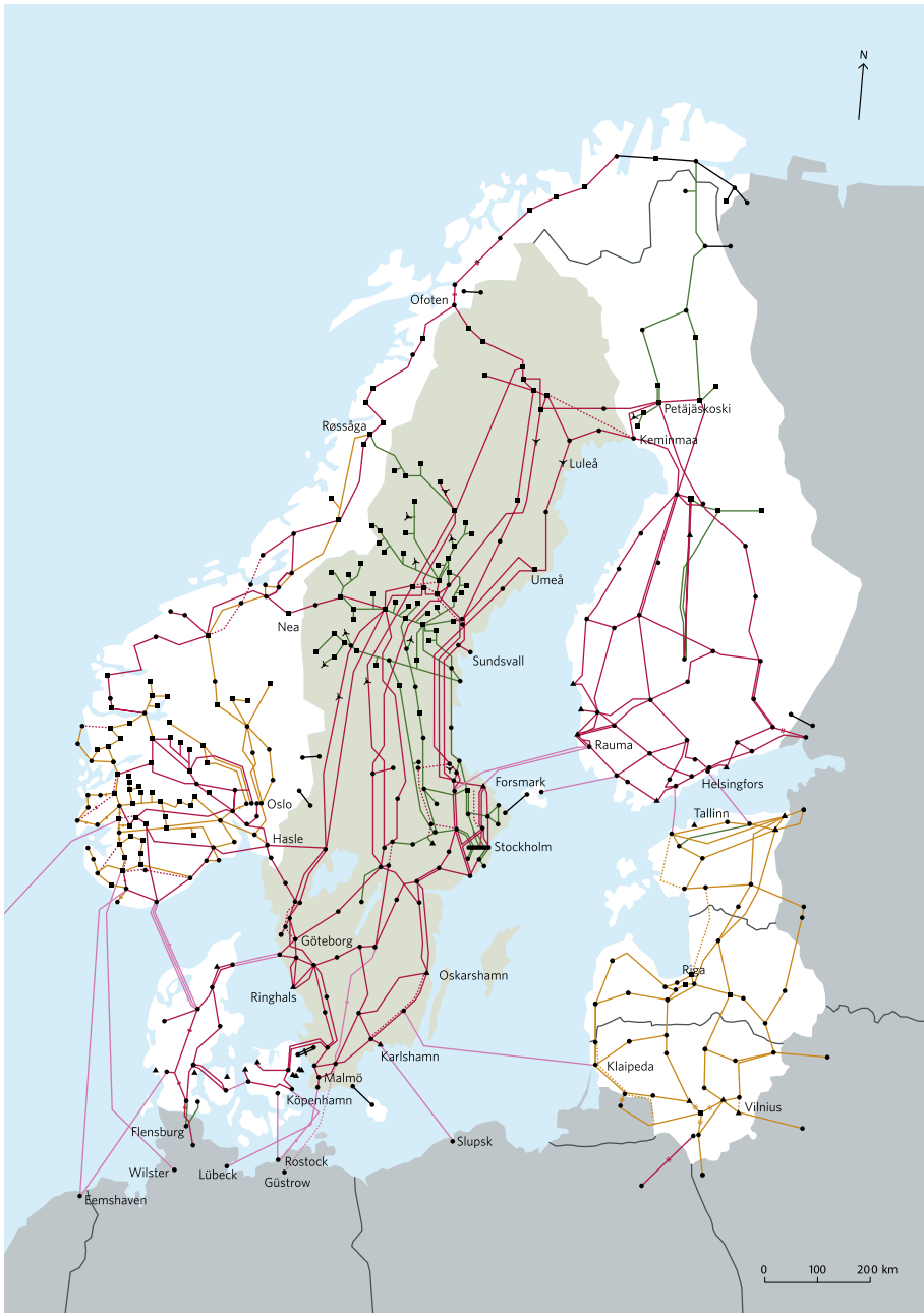
Figure 3.10: Map of the Nordic transmission system. This includes the Nordic synchronous area (Sweden, Norway, Finland, and Eastern Denmark) and parts of the continental European system (Estonia, Latvia, Lithuania, and Western Denmark)[66].
