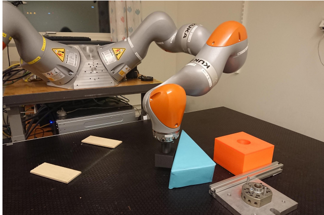
Figure 1.1: The robot setup used for the experiments. Wooden boards indicate the start location for the push task. The goal is the corner between the fixture and the box with the hole for the peg task.
