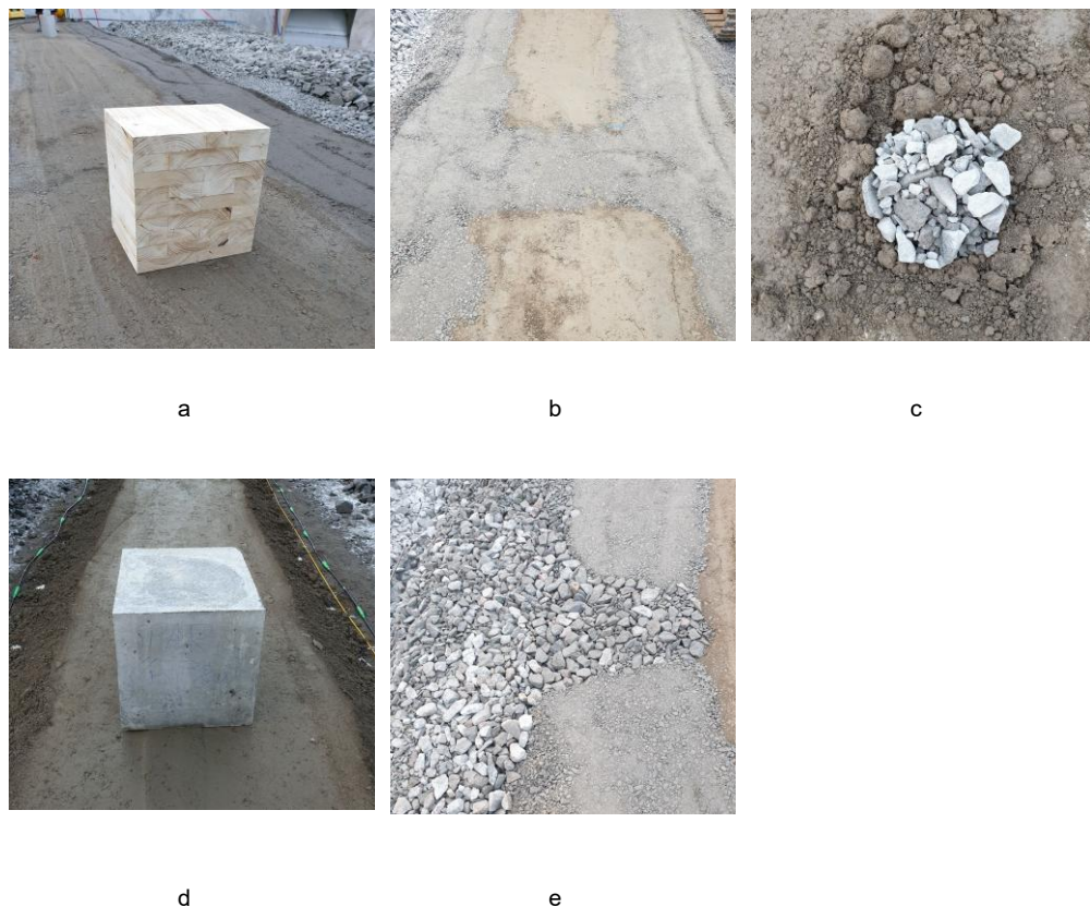
Figure 17. The defects incorporated inside the core and filter; a) The cavity in the core (Defect No. 1); b) The horizontal permeable zones in the core (Defects No. 2 and 5); c) The vertical loose zone in the core (Defect No. 3); d) The lump of concrete in the core (Defect No. 4); e) The filter defect (Defect No. 6) (Lagerlund et al., 2022).
