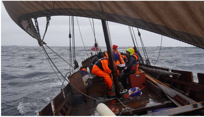
Fig. 4. Experimental insights into Greenland Norse seafaring capabilities: example of a larger expeditionary sailing vessel. This is a Norwegian fembaring, a direct descendant of the Norse clinker tradition used in Greenland (Vestfjord, northern Norway, May 2022). Only these larger sailing ships, owned and sponsored by richer farmers and elites, would have been capable of reaching the North Water Polynya during single-summer expeditions. One major risk was becoming trapped in the expanding late-summer pack ice, forcing the crew to overwinter en route, as evidenced by the Kingittorsuaq runestone (Fig. 5) carved during the Spring, and dating to ca. 1250 to 1300 CE (see Supplementary Text). Photo: G.J.
