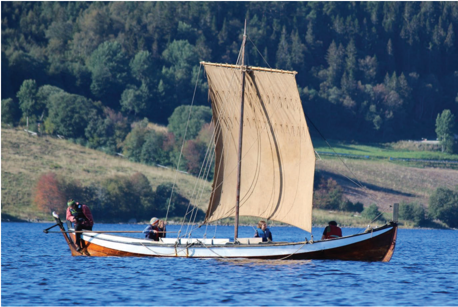
Fig. 3 Continuities in boatbuilding traditions from the Viking Age are evident in the shape and rig of this fyring , a smaller type of Åfjord boat similar to the vessels associated with non-elite Viking Age farmsteads. Image courtesy of Tora Heide
