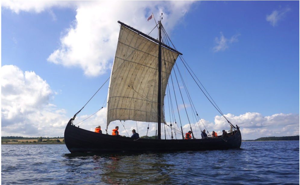
Supplementary Figure S2. Larger ‘expeditionary’ vessel employed by Greenland Norse. This modern example is a compact, clinker-built, square-rigged cargo vessel based on the design of the Skuldelev 1 wreck, which was built in western Norway c.1030 CE. Norse Greenlanders could only undertake walrus harvesting expeditions to the North Water Polynya in these larger sailing vessels, which were owned by wealthier farmers and elites, adding an important socio-political dimension to Late Period exploitation strategies. Photo: Greer Jarrett.
