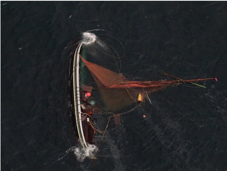
Fig. 6 Katabatic winds are caused by thermal differences between sea-level and high-altitude areas in close proximity to each other, and can be extremely dangerous when sailing near land. In the summer of 2023, a katabatic gust caused this fembøring to capsize off the coast of Kunna. Image courtesy of HRS Nord-Norge (No. 330 Squadron RNoAF)
