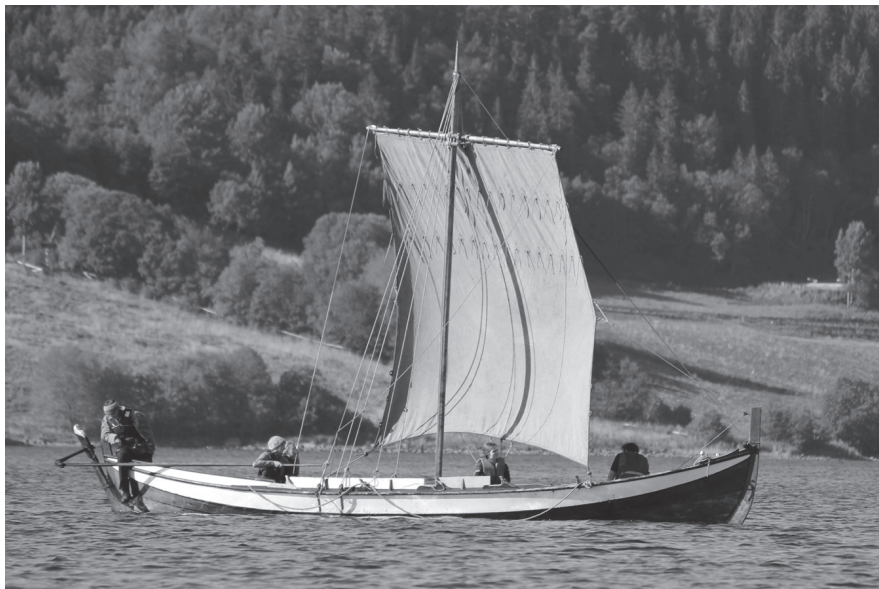
Figure 12.4. A traditional Norwegian boat built following the Åfjord tradition. Rissa, Trøndelag, September 2021. Just like the boats of the Viking Age, Åfjord boats are built frame-first and rigged with a square sail. Image courtesy of Tora Heide.
