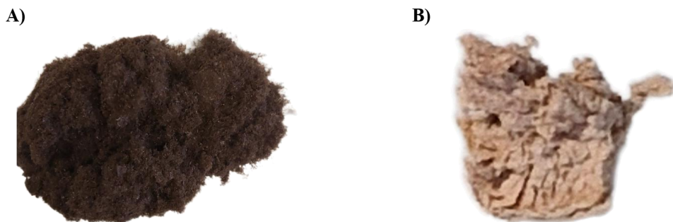
Figure 7. A) Freeze-dried hemicellulose fraction of cañihua seeds after alkaline extraction. B) Freeze-dried cellulose fraction after hemicellulose extraction of cañihua seeds.
