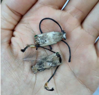
Figure 3. Two multisensor data loggers retrieved from thrush nightingales after one year of deployment. These devices recorded detailed data on migratory behaviour throughout the annual cycle. Photo: the author.
