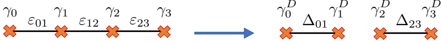
Figure 38: Graphical representation of the second move of MBS diagrammatics, which splits up a hybridization chain of four MBS into two pairs of hybridized MBSs.
