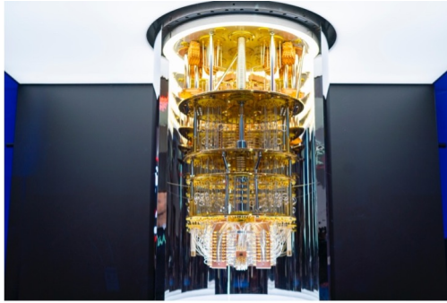
Figure 2: One of the IBM quantum computers. Most of the machine is a cryostat, providing several layers of cooling. The actual chip containing the qubits is the black dot sitting at the bottom of the setup. The figure was taken from [13].
