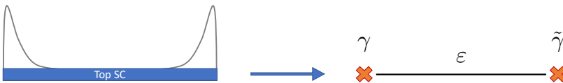
Figure 13: Effective representation of a topological subgap state (gray line, left) via two zero-dimensional MBS operators (orange crosses, right).
