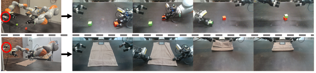
Figure 5: Real-world experimental setup and task progression. (Left) The dual-arm manipulation environment for the Stack Block Two (top row) and Towel Folding (bottom row) tasks. The wrist and head cameras are not used for both task, the red circle indicates the single scene camera which provides visual observation input for the models. (Right) Key terminal stages of the tasks viewed from the perspective of the scene camera. These stages correspond to the bottleneck evaluation milestones (e.g., picking, placing, and folding).
