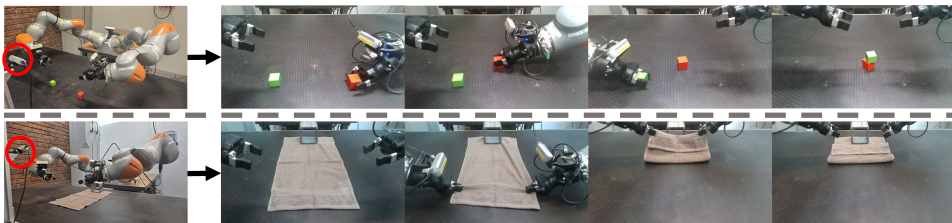
Figure 21: The two real-world robot experiments. Top: block stacking. Bottom towel folding. The red circles in the leftmost pictures highlight the camera used to view the scene.
