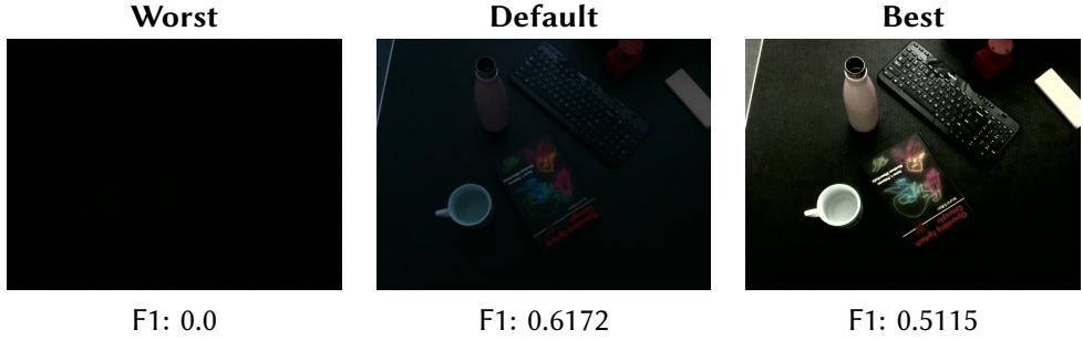
Figure 9: Example where parameter optimization resulted in worse performance in object detection. Left: lowest log-likelihood. Center: default parameters. Right: highest log-likelihood.
