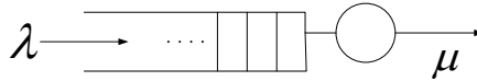
Figure 3. A single server queue with mean arrival rate \lambda and mean service rate \mu .
