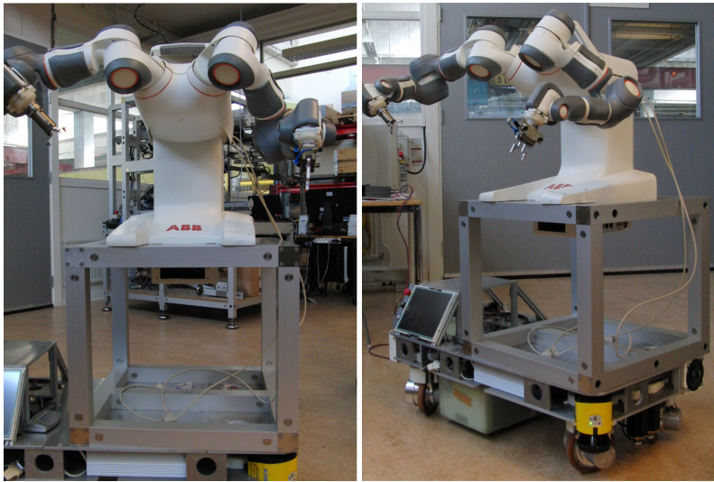
Figure 1.1 Mounting an industrial manipulator on a mobile robot platform offers flexible and cost-efficient assembly solutions. Because the industrial manipulator’s work space is now dynamic, the setup also demands more knowledge about the environment.
