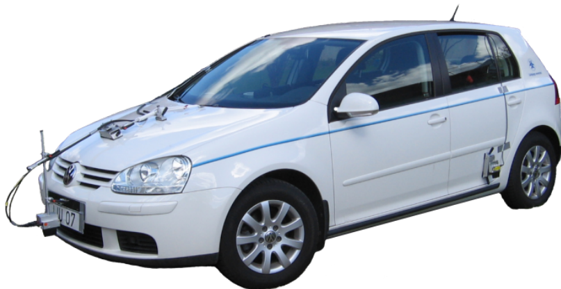
Figure 9.4 The vehicle testbed used in the experiments. The velocity sensor is placed at the front end, aligned with the longitudinal axis. The roll and pitch angle sensors are situated at the front end and in front of the rear wheels. The vehicle was also equipped with a GPS receiver during the experiments.
