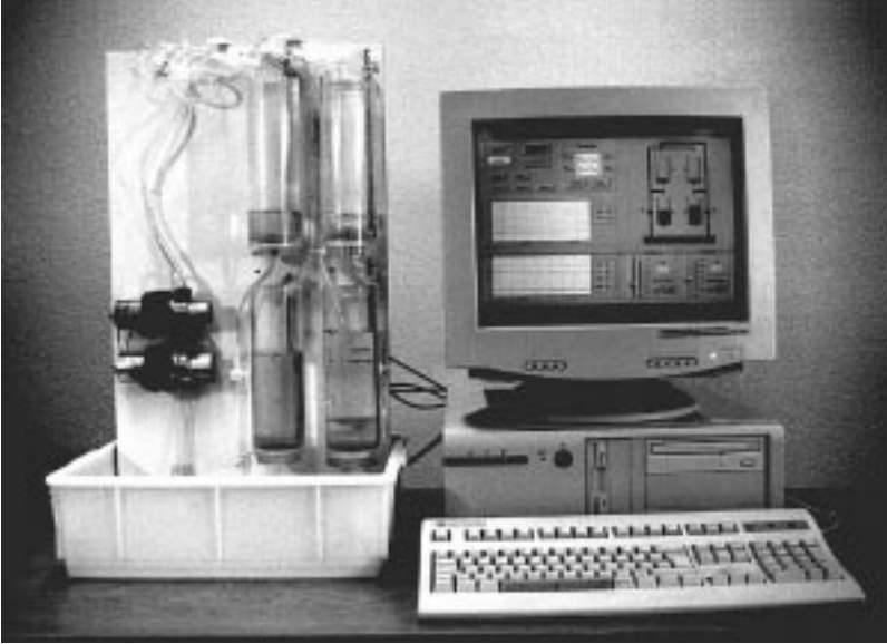
Figure 1. The quadruple-tank laboratory process. The water levels in the lower two tanks are controlled with the help of two pumps.
