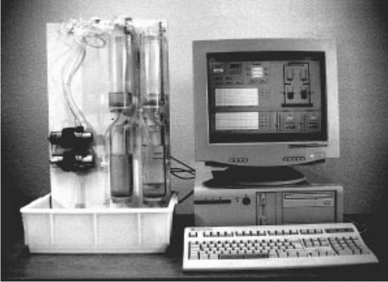
Figure 1. The quadruple-tank laboratory process shown together with a new controller interface running on a Pentium PC.
