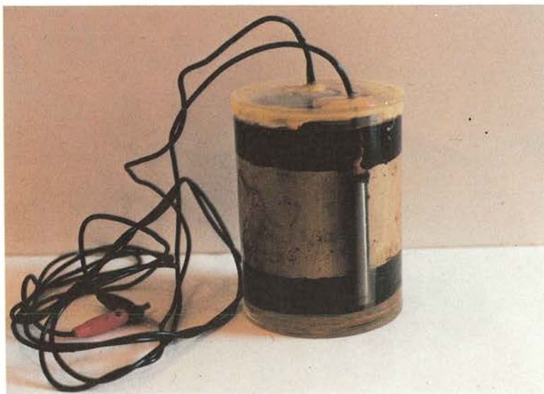
Photo 40. The process of corrosion stopped by repassivation or lack of O_2 . Cathode cast into concrete, anode in waterfilled space. Exposure time 5 years.
