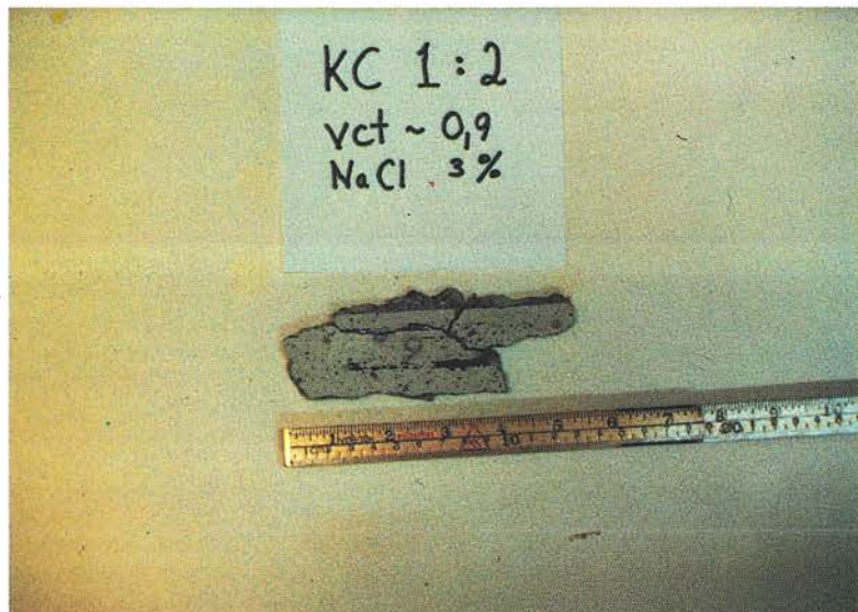
Photo 11. The concrete cover also showed clear marks of a corrosion attack.
