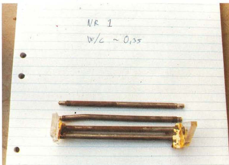
Photo 24. Anodic metal surfaces have received faint brown discolouring. Cell No. 1, in Series 2.
