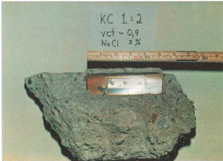
Photo 9. Embedded corrosion cell after concrete had been chipped away.
