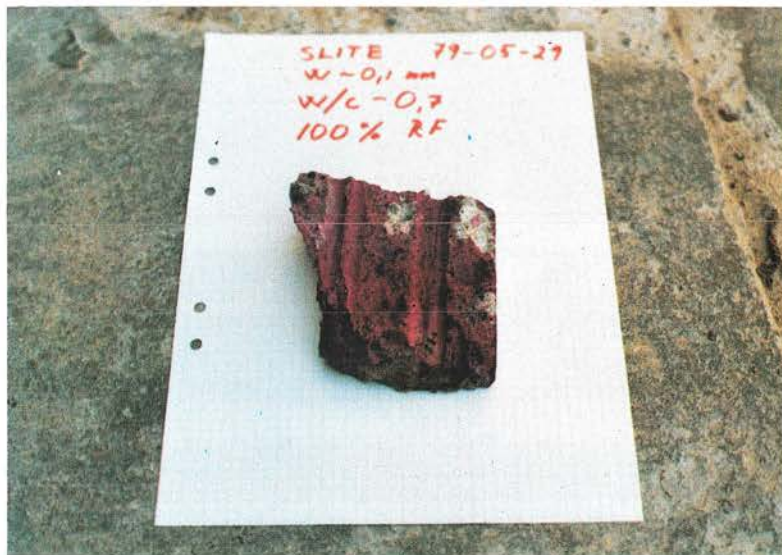
Photo 41. Realkalization has occurred in crack zones after increased relative humidity in the environment. Phenolphthalein test is positive.
