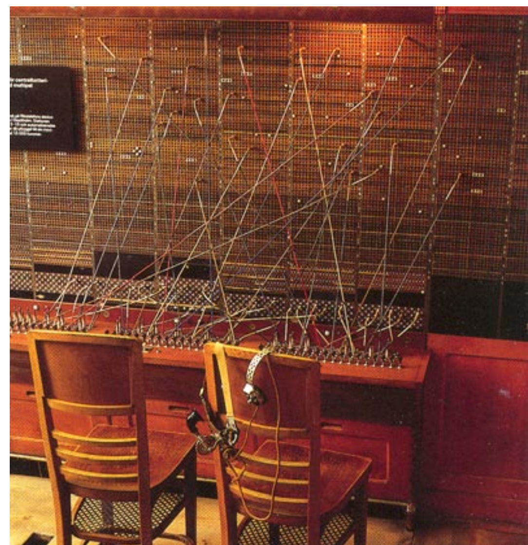
Fig. 30 Image of point-to-point connection in a classic telephone system.
