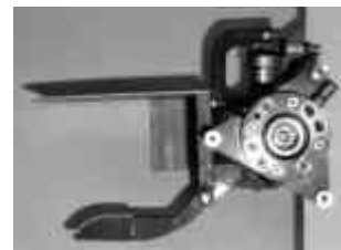
Figure 4.9 Top view of the RAID1 book gripper
