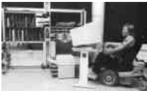
Figure 4.3 RAID workstation (prototype) with moving robot, framework with bookshelves, and storage for diskettes, documents and peripherals, such as a printer, etc. Photo: Helena Alvesalo.
