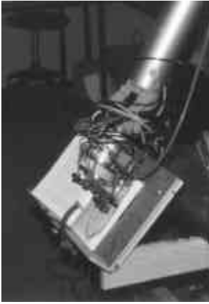
Figure 4.29 The operation of the page turner was tested at high speeds using a fast industrial robot (IRb1000 from ABB).
