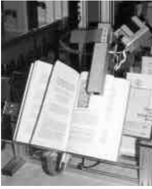
Figure 4.41 The RAID1A page turner is capable of moving books to and from the readerboard as well as turning pages. In this way, the time-consuming change-over from book gripper to page turner is avoided.
