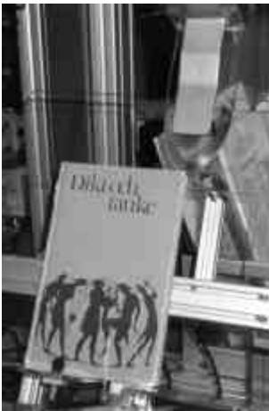
Figure 4.48 When the robot has measured the thickness, height, and width of the book it places the tip of the end-effector at the upper right-hand corner of the book to confirm that the measurement is correct.
