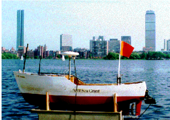
Figure 4: The USV Artemis, developed by MIT in 1993 [23].
