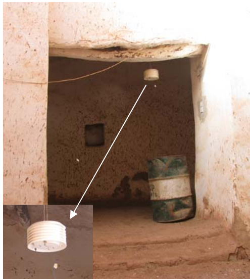
Figure 5.5 Outdoor temperature measuring loggers in Balat.
