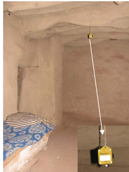
Figure 5.6 Indoor temperature measuring loggers in Balat.
