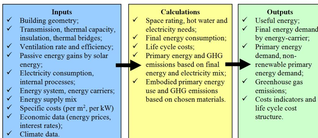
*Fig. 1 Simplified model of used methodology*
