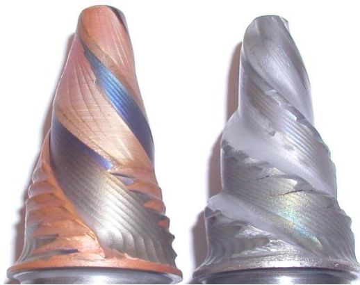
Figure 4-19. Probe with 17 mm MX (left) used for one full cycle, and a full MX probe (right) used for one full cycle plunging into a cylindrical pilot hole.
