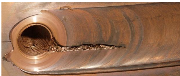
Figure 4-1. Visible wormhole during lid weld at TWI.
