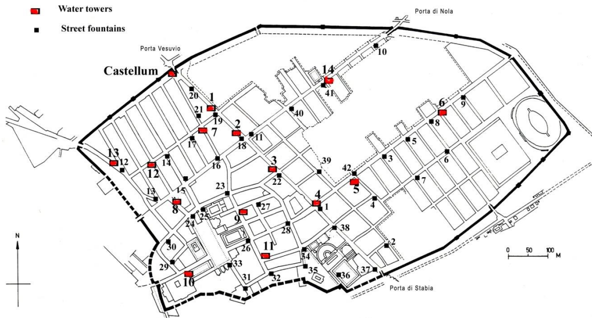
Figure 3.1. Location of street fountains and water towers. The towers are numbered 1-14 and are indicated in red, while the fountains are in black and numbered 1-42. Drawing by author.
