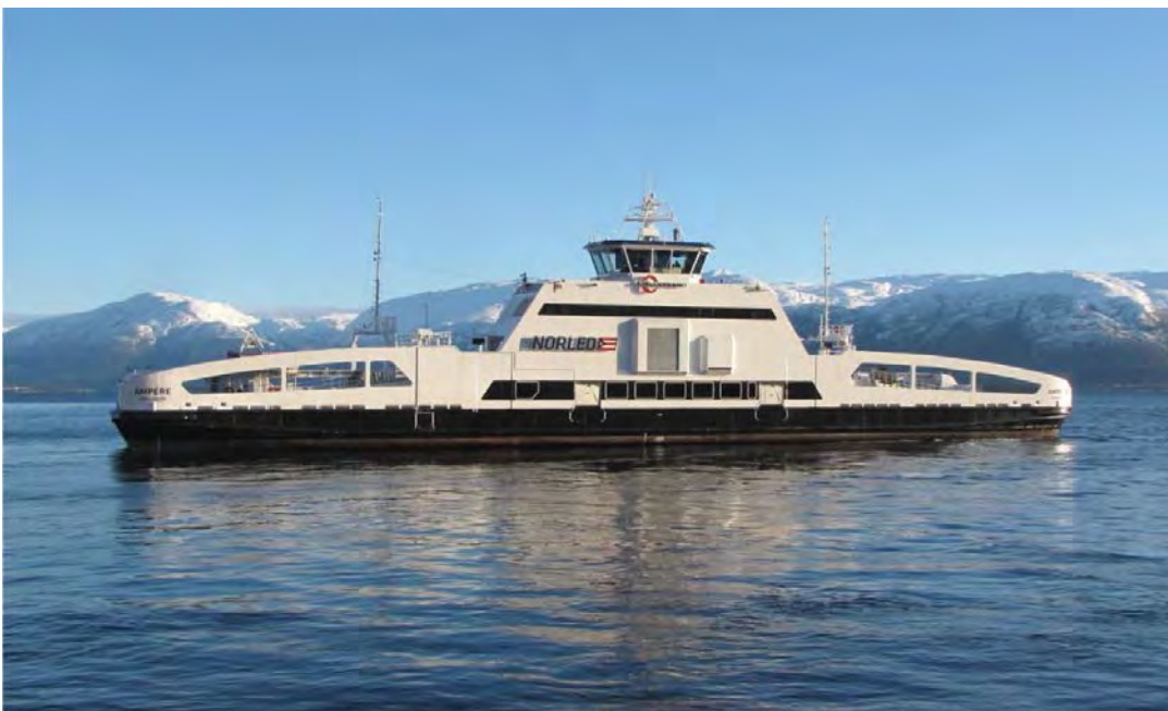
Figure 11 The battery electric ferry M/F Ampere . Source: Fjellstrand
