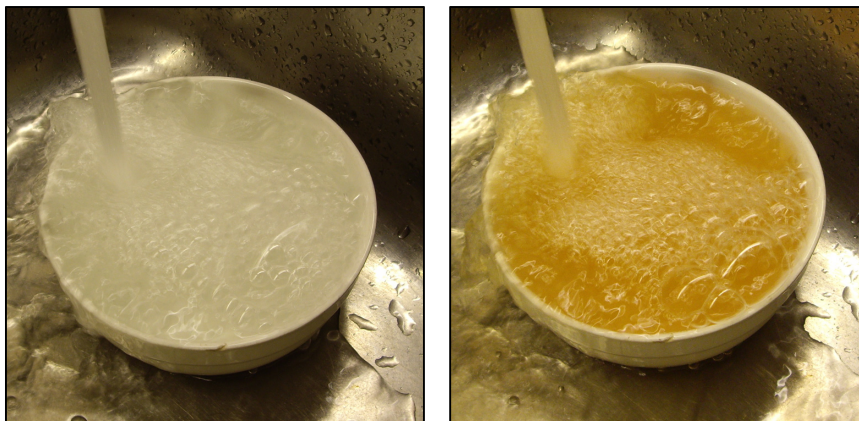
Figure 5. Photograph of flowing water in a kitchen sink taken during sampling while red water occurred.
