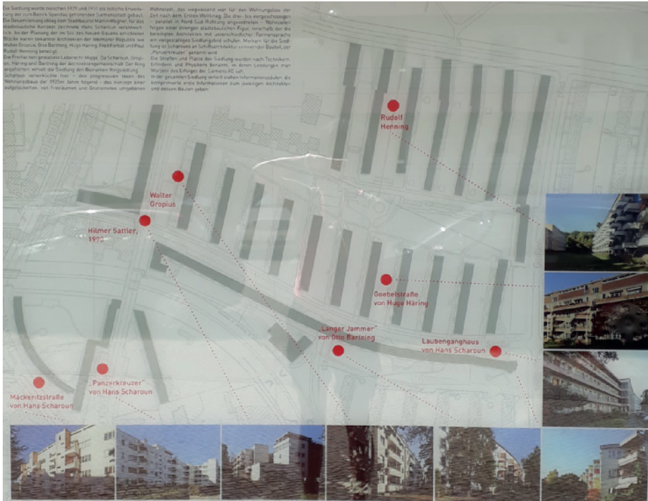
Figure 1.3 A site plan of the housing estate Siemenstadt (1929–1931), showing the open arrangement and equal spacing between the rows of buildings (designed by Hans Scharoun, Walter Gropius, Otto Bartning, Hugo Häring, Paul Rudolf Henning, and Fred Forbat). (Photograph taken by the author at the information point in the estate.)
