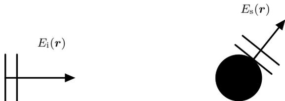
**Figure 37:** An incident wave impinges on a small scatterer generating a scattered field.
