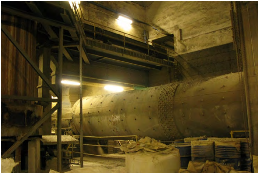
Figure 23. Rotary kiln at the Cementa plant in Degerhamn, Öland, Sweden. (From the picture archive of the Department of Occupational and Environmental Dermatology, photographer unknown)
