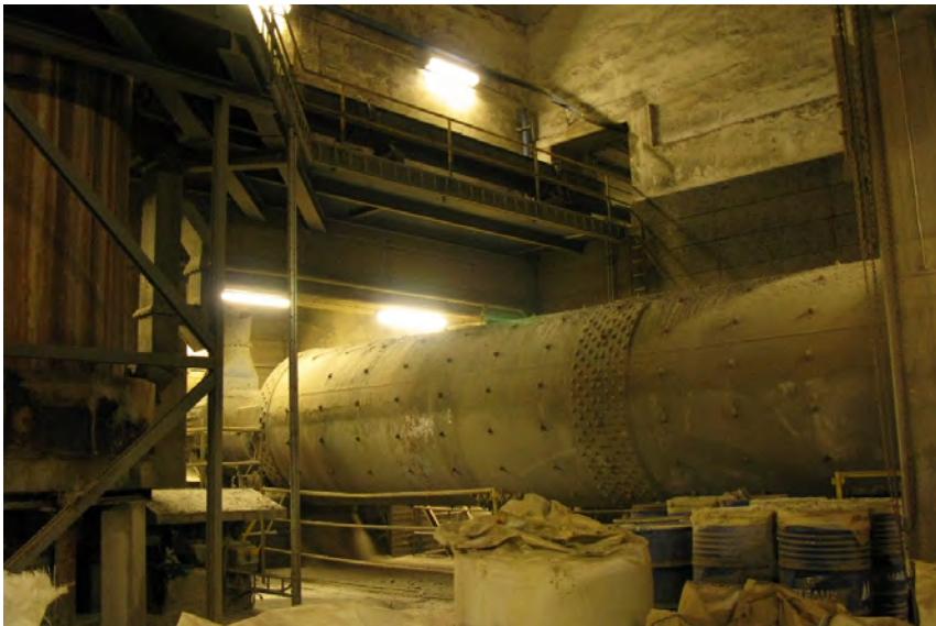
Figure 23. Rotary kiln at the Cements plant in Degerhamn, Öland, Sweden. (From the picture archive of the Department of Occupational and Environmental Dermatology, photographer unknown)
