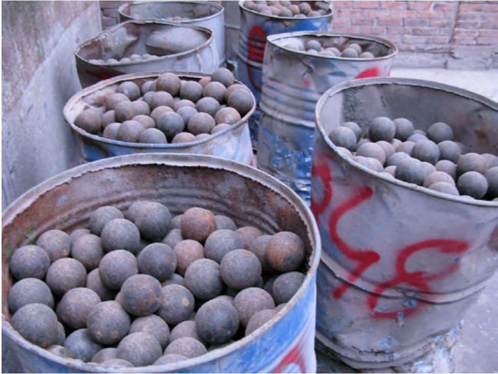
Figure 26. Metal balls used to grind cement clinker to cement powder. (From the picture archive of the Department of Occupational and Environmental Dermatology, photographer unknown)
