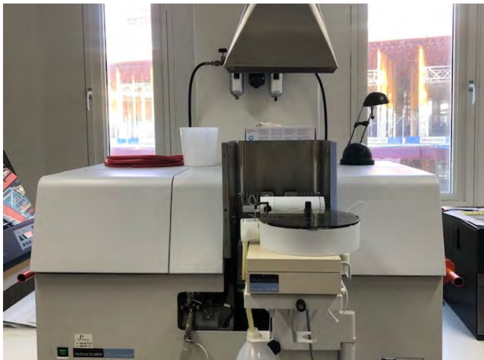
Figure 33. The AAAnalyst 800 at our laboratory.
