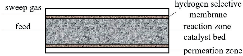
Figure 2.6: Hydrogene selective membrane reactor schematic.
