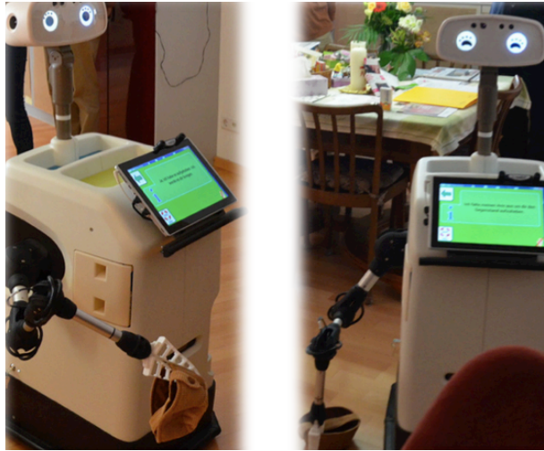
Figure 10: The assistive robot picking up an object from the floor
