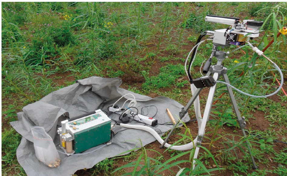
Figure S1. Experimental setup of leaf chamber system. To the right on the top of the tripod, the leaf chamber is attached and connected to the portable photosynthesis system (LI-6400) to the left. BVOC-sampling was done by taking a sub-sample of 200 ml/min of air leaving the leaf chamber using adsorbent tubes filled with Tenax TA and Carbograph with a small flow regulated pump.
