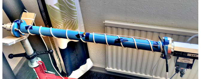
Fig. 1. Rigid coaxial line with directional coupler (to the right) used in the phase-reference distribution system at ESS. Sensors for surface measurements of the temperature and a heating cable wound around the outer copper tube have been mounted on the coaxial line. The complete phase-reference line and directional couplers are then insulated (see Fig. 7).
