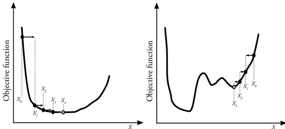
**Figure 3. Graphical illustration of the gradient descent method**
