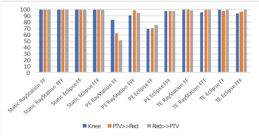
**Figure 9.** Gamma pass rates from Delta4 measurements of VMAT plans generated in Eclipse and RayStation, using FF and FFF beams. Plans from three Pareto levels: static phantom and with two simulated motion patterns.
