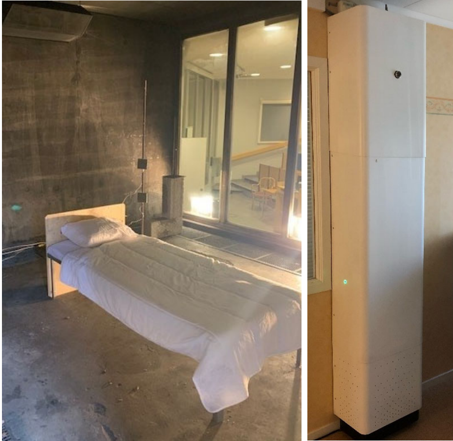
Figure 2 – Picture of a typical experimental set-up (left) and a picture of the Q-fog (right). Note that in the actual experiments, the unit was placed outside the room and only the nozzle placed in the room to prevent contamination of the unit.
