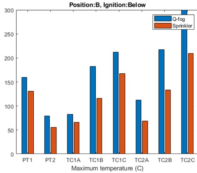
Figure 14 – Maximum temperature during the SB2 and QB2 tests.
