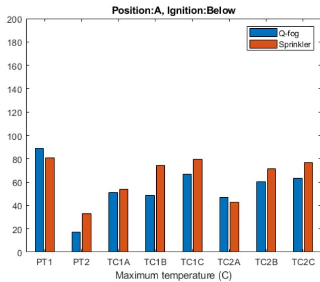
Figure 8 – Maximum temperature during the SA2 and QA2 tests.
