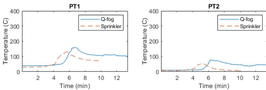
Figure 12 – Plate thermometer temperature for the SB2 and QB2 tests.
