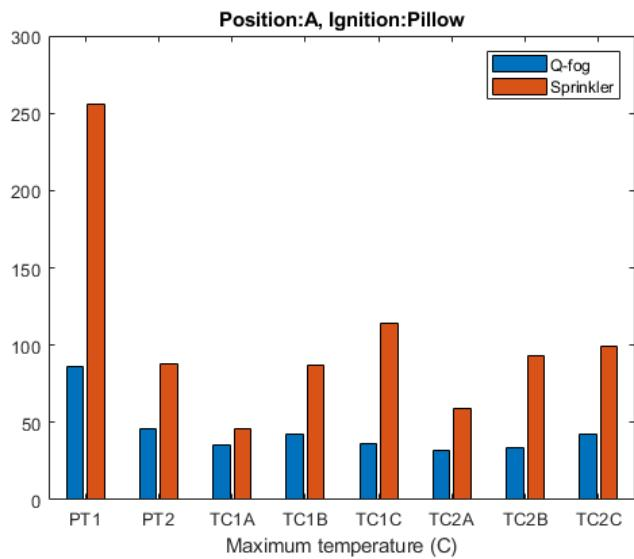
Figure 5 – Maximum temperature during the SA1 and QA1 tests.
