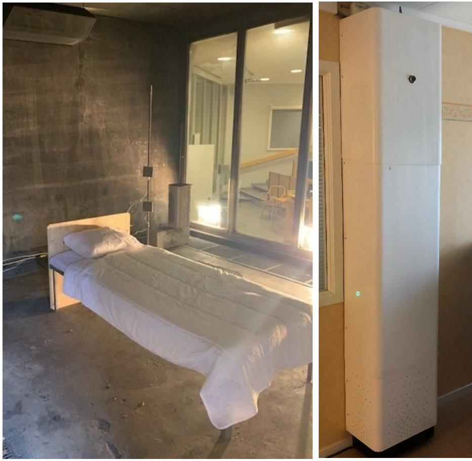
*Figure 2 – Picture of a typical experimental set-up (left) and a picture of the Q-fog (right). Note that in the actual experiments, the unit was placed outside the room and only the nozzle placed in the room to prevent contamination of the unit.*
