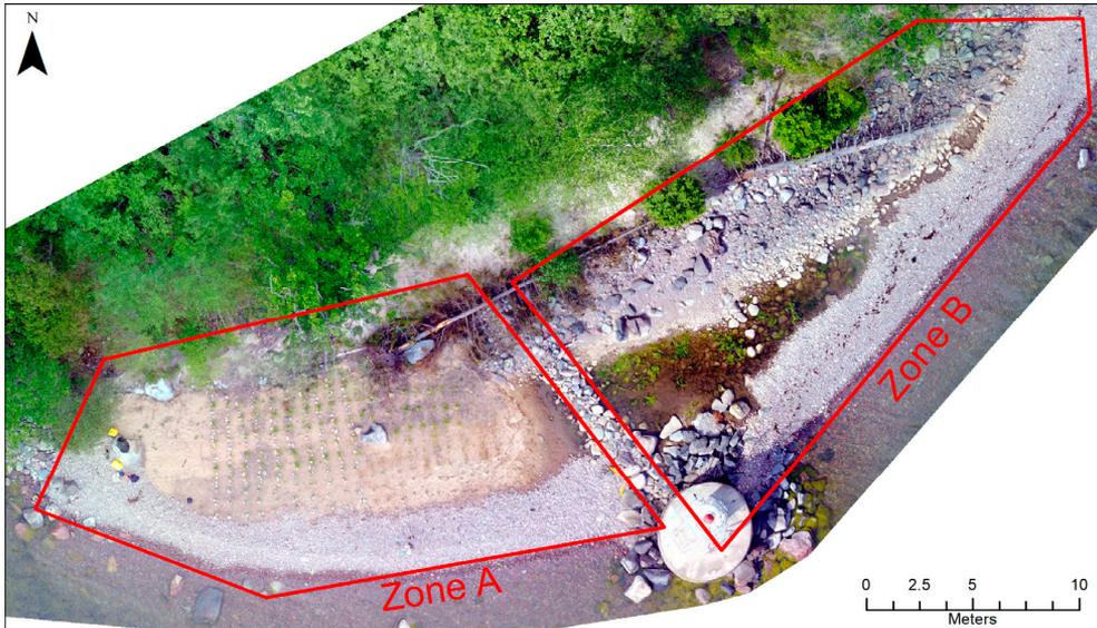
**Figure 4-3.** Aerial photograph of Staboudde taken one month (June 2016) after completion of the nature-based erosion protection. Zone A shows the zone with a backshore landward of the sill. Zone B is the zone without a backshore. (Photo by Mats Öberg, SGI)
