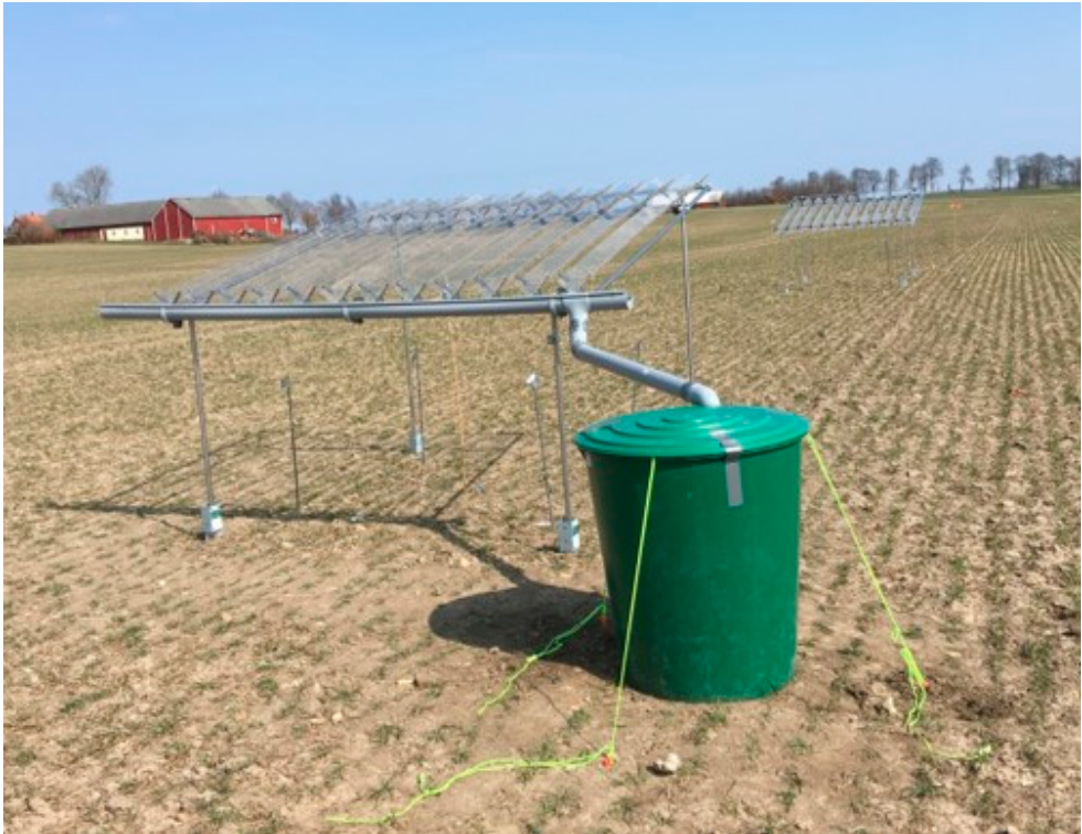
Figure 3: Drought manipulation experiment in Paper II and III . Fixed location, partial rainout-shelters to impose a drought by reducing the 65% of the precipitation (Roof treatment, R) across the spring and summer winter wheat growing season. Photo: María Ingimarsdóttir.
