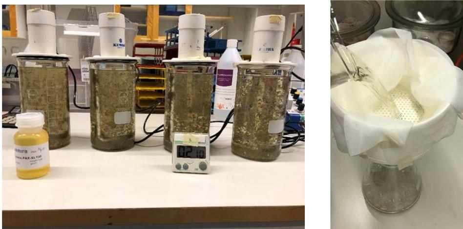
**Figure 6.** Jar tests with Al- and Fe-based coagulants and anionic polymer (left) and the separation of flocs on a microfilter cloth (right).
