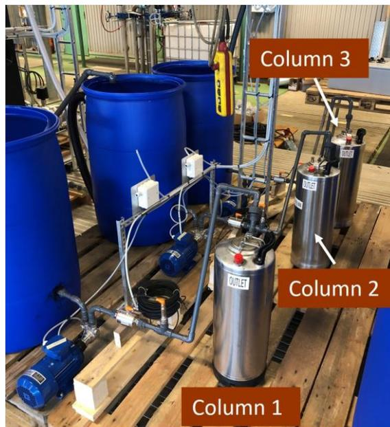
**Figure 11.** Columns containing sand and GAC. Column 1 contained GAC for treatment downstream of CEPT, microsieving and DMF (UF). Column 2 contained sand and column 3 contained GAC. Column 2 and 3 were connected in series (sand first) for treatment downstream of the WWTP.
