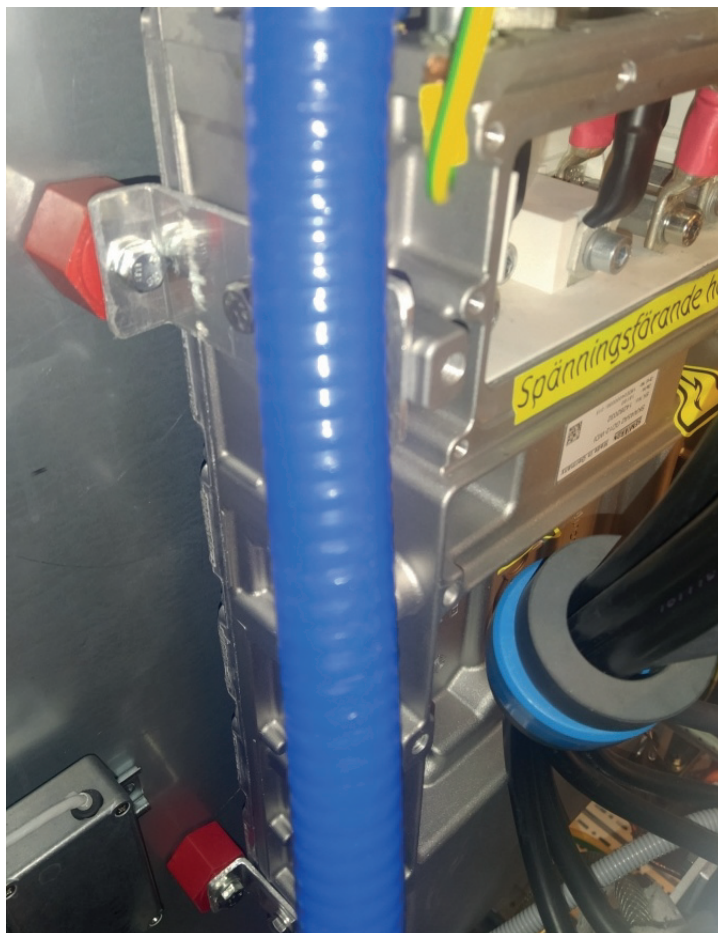
Figure A.4: The mounting of the traction converter in the electrical cabinet. The red mounting points are isolators. The blue hos in the foreground the coolant supply to the converter.
