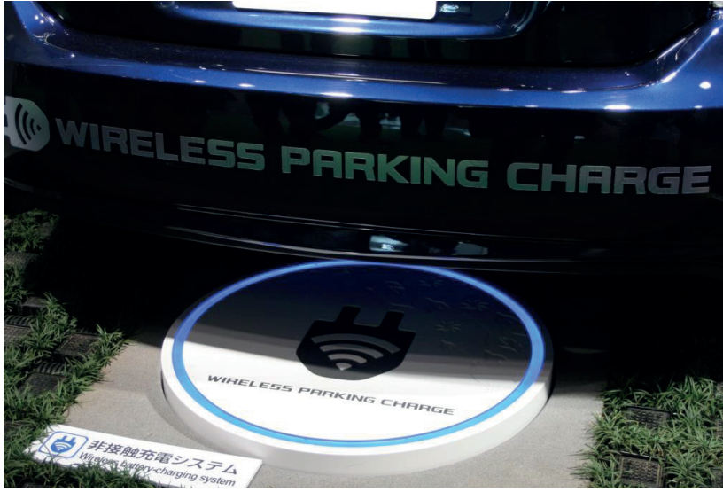
Figure 1.4: An inductive charging pad [14].
