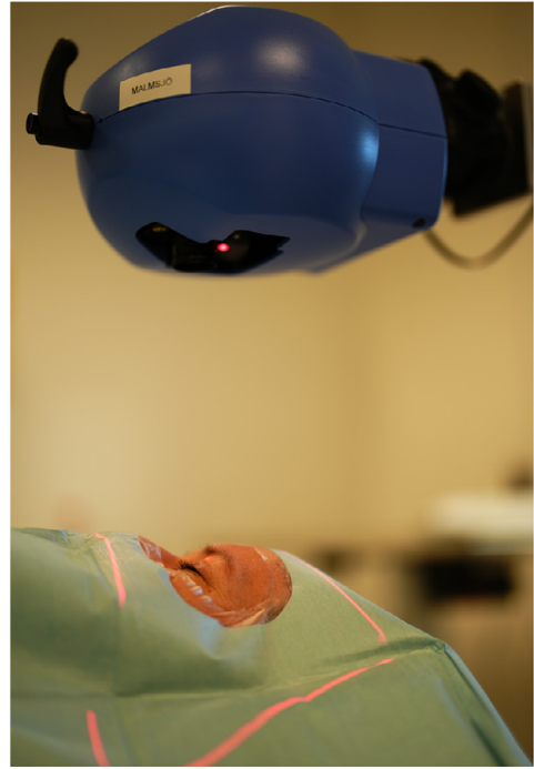
Figure 6. Photograph showing the PeriCam equipment for perfusion monitoring during surgery. The visible red laser light (650 nm) seen in the photograph is used for positioning. (Photograph by Rafi Sheikh)
