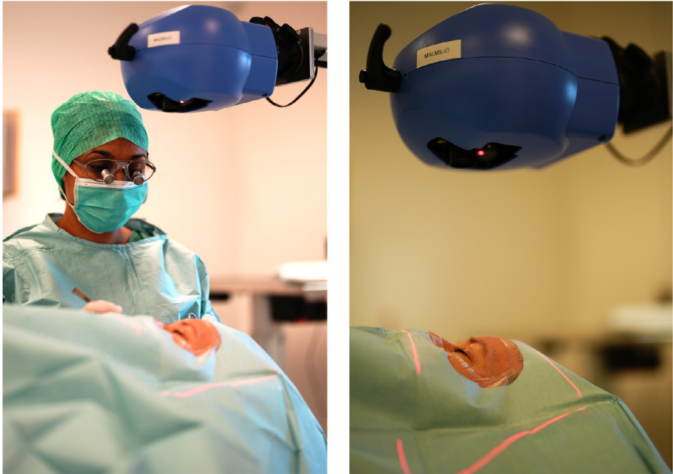
Figure 6. Photograph showing the PeriCam equipment for perfusion monitoring during surgery. The visible red laser light (650 nm) seen in the photograph is used for positioning. (Photograph by Rafi Sheikh)
