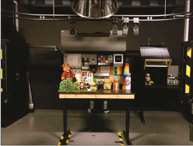
Figure 5. Image laboratory used to determine characteristics related to the camera and the scene.
