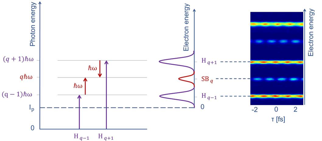
**Figure 4.2: Principle of RABBIT.** Sideband  $SB_q$  appears in the photoelectron spectrum as a result of the  $H_{q-1} + IR$  and  $H_{q+1} - IR$  transitions. The modulation of the sideband signal with the XUV-IR delay  $\tau$  encodes information about the atomic potential.
