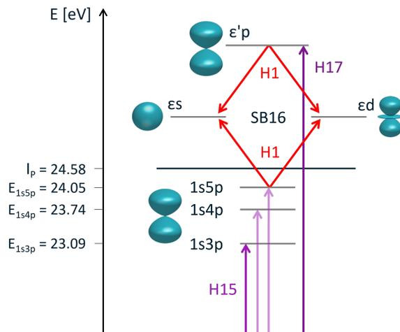
**Figure 5.10: Experimental scheme.** H15 is tuned into resonance with the  $1snp$ ,  $n=3-5$  Rydberg states of He, whilst H17 ionises the atom. A weak H1 (fundamental) signal is combined with the harmonics, creating SB16 through  $s$  and  $d$  angular momentum channels.
