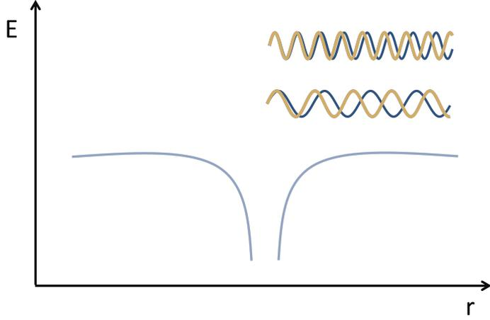
**Figure 5.1: Electron wavepacket phase.** As it moves away from the nucleus, the photoelectron wavepacket scatters off its attractive potential. This results in a phase shift between the energy-dependent phase the wavepacket acquires (yellow) compared to that of a wavepacket outside any field (blue).
