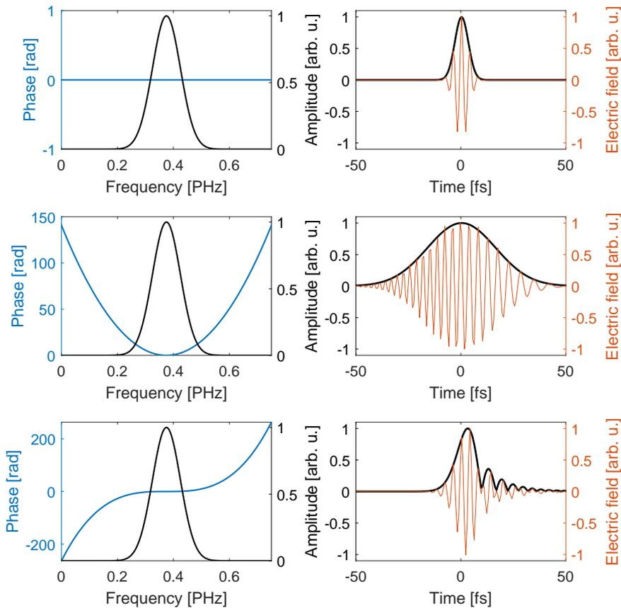
**Figure 3.1: Impact of spectral phase on pulse shape and duration.** Left column: spectrum (black) and spectral phase (blue); right column: pulse amplitude in time (black), electric field (red). From top to bottom row: Fourier transform limited pulse, pulse with GDD only, pulse with TOD only.
