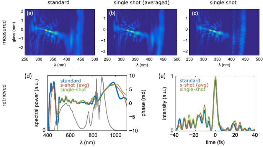
**Figure 3.13: Comparison between single-shot and sweeping d-scan performance.** D-scan spectrograms produced using (a) standard sweeping d-scan (fused silica wedges), (b) single-shot d-scan while integrating over about 15 pulses, (c) single-shot d-scan applied to one individual pulse. The retrieved spectral phase (d) and temporal profile of the pulses (e) are in excellent agreement. Grey line in (d): spectrum of the studied HCF-broadened pulse. Adapted from Article II.
