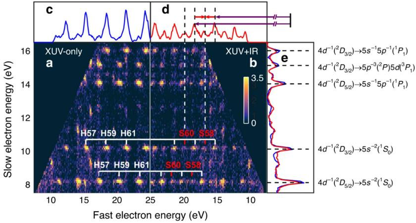
**Figure 5.7: Two-electron coincidence map.** Coincidence map for a) XUV only, b) XUV+IR. Projections on the fast electron energy axis for c) XUV only and d) XUV+IR. The applied RABBIT scheme is indicated by violet (XUV) and red (IR) arrows. Projections on the slow electron energy axis (e) for XUV-only (blue) and XUV+IR (red), showing peaks originating from different Auger channels. Taken from Article V.
