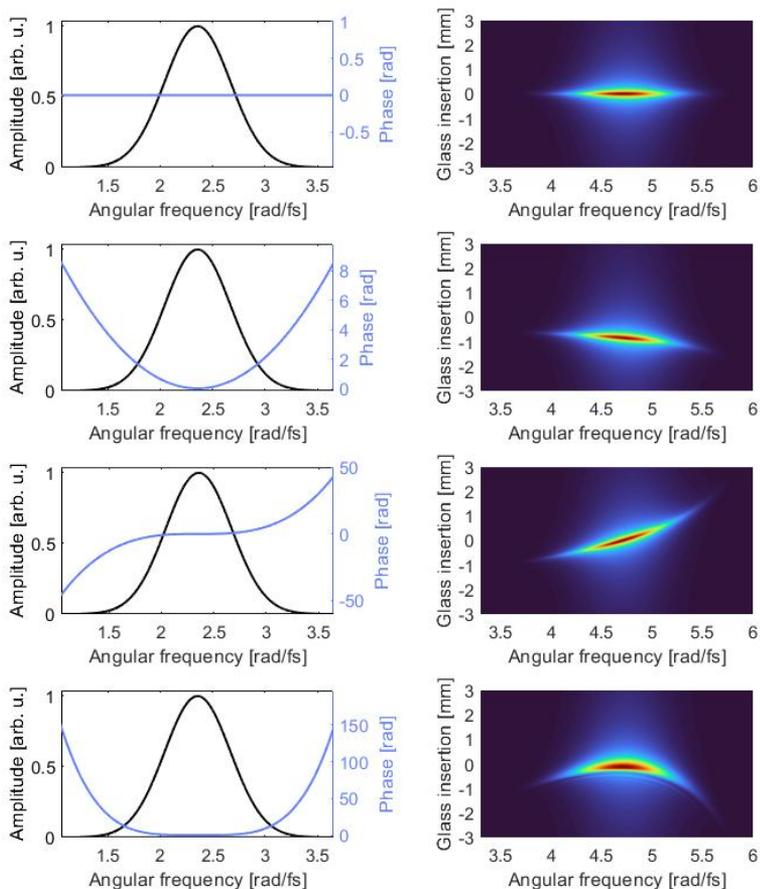
**Figure 3.11: D-scan traces of pulses with different dispersion orders.** Left: spectrum and spectral phase of the pulse; right: corresponding simulated d-scan traces. From top to bottom: Fourier transform limited pulse, pulse with second, third, and fourth order dispersion.
