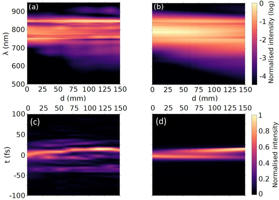
**Figure 3.18: Pulse evolution along the filament length.** Top: spectral evolution, bottom: temporal evolution. Left: interpolation from measurements at 9 points along the filament length, right: calculations.
