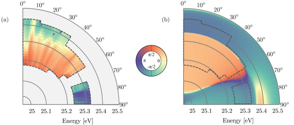
**Figure 5.12: Angle-and-energy-resolved phase around the  $4p$  resonance.** A phase jump in energy of approximately  $-\pi$  rad is observed at resonance, and in angle around  $65^\circ$ . (a) VMIS data, areas with low signal-to-noise ratio filtered out. (b) theoretical calculation. The colour scale is common for the two panels.
