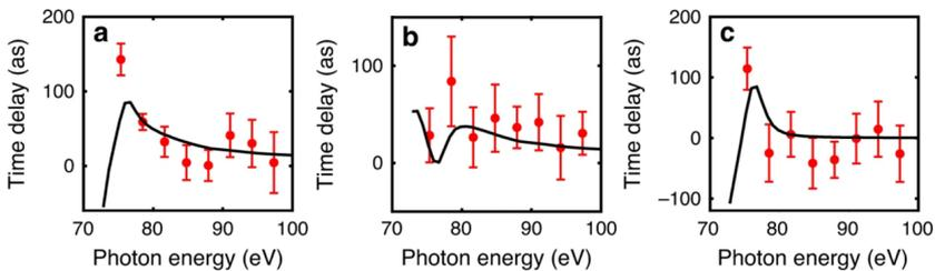
**Figure 5.8: Photoemission time delays in Xe.** Time-delay differences: a)  $\tau_A[\text{Xe}(4d_{3/2})] - \tau_A[\text{Ne}(2p)]$ , b)  $\tau_A[\text{Xe}(4d_{5/2})] - \tau_A[\text{Ne}(2p)]$ , c)  $\tau_A[\text{Xe}(4d_{3/2})] - \tau_A[\text{Xe}(4d_{5/2})]$ . Red: experimental data, black: calculations. Adapted from Article V.
