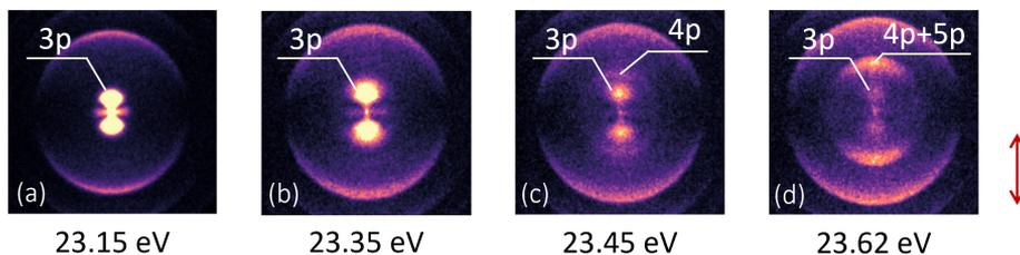
**Figure 5.11: VMIS images of SB16 upon tuning H15 across Rydberg states in He.** Energy of H15 is indicated below each image. (a) and (b) only 3p resonance visible; (c) 3p and 4p resonances; (d) mostly 4p and 5p resonance populated. Central part of non-inverted VMIS images only. The red arrow indicates the polarisation direction.
