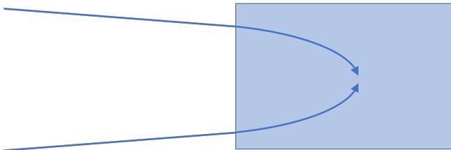
**Figure 3.6: Schematic illustration of self-focusing.** The light-induced transverse refractive index gradient has the same effect as a focusing lens. If diffraction effects cannot prevail, self-focusing leads to beam collapse towards the centre.
