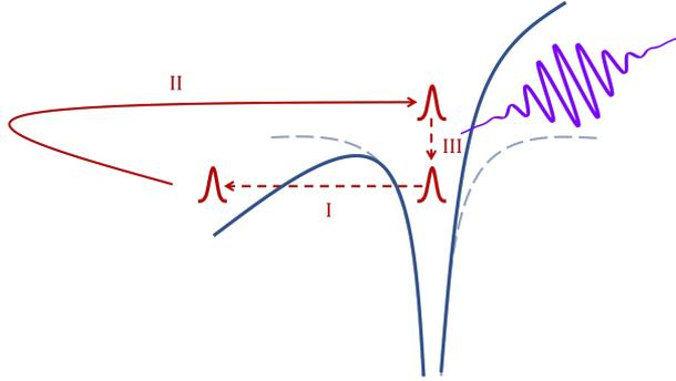
**Figure 2.2: Three-step model.** An electron is (I) liberated via tunnel ionisation when the external field lowers the atomic barrier, (II) accelerated by the same field, (III) recombined with the parent ion as the field sign reverses. Upon recombination, energy equal to the sum of electron kinetic energy and  $I_p$  is released in the form of a photon.
