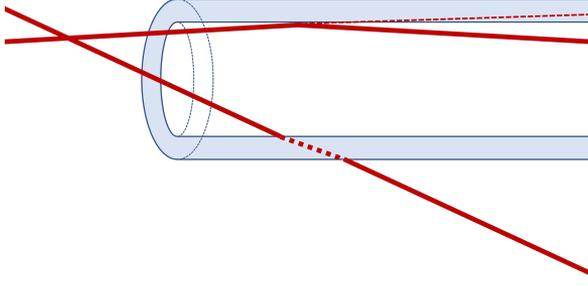
**Figure 3.7: Hollow-core fibre operation principle.** Light is guided through the gas-filled core via grazing incidence reflections with minor losses. Rays entering the fibre at larger angles suffer high reflection losses.
