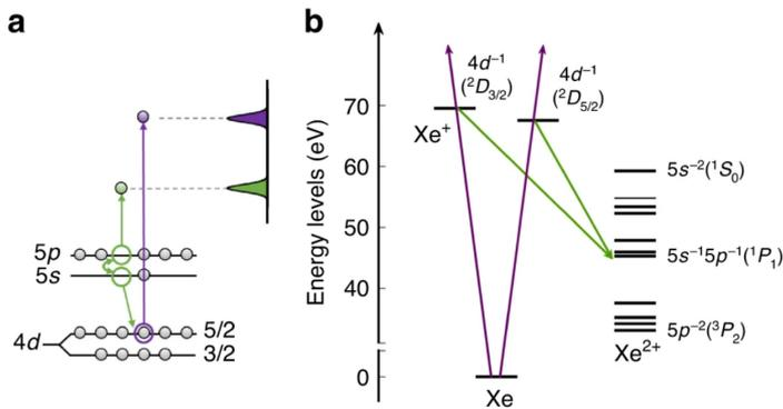
**Figure 5.6: Xe 4d ionisation scheme.** a) Direct photoionisation (violet) and Auger decay processes (green) initiated by absorption of harmonic radiation; b) Xe energy diagram detailing the direct and Auger ionisation paths (violet and green, respectively). Taken from Article V.
