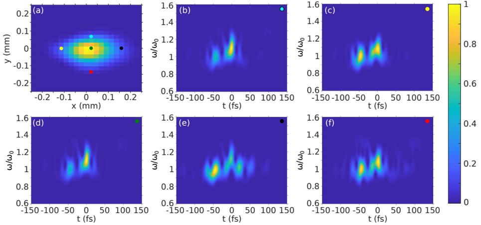
**Figure 3.20: Spatially resolved time-frequency analysis.** The beam profile features considerable pulse form variations. (a) Cross-section of the beam, (b-f) time-frequency representation of the pulse corresponding to the selected pixels.
