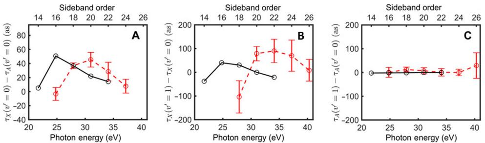
**Figure 5.5: Relative molecular time delays in N2.** Time-delay difference between (A) X and A states for  $v'=0$ , (B)  $v'=1$  and  $v'=0$  vibrational levels in the X state, (C)  $v'=1$  and  $v'=0$  vibrational levels in the A state. Red: experimental data, black: calculations. Adapted from Article IV.
