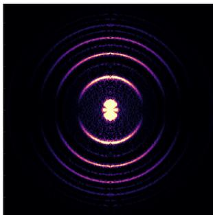
**Figure 4.8: Iteratively inverted VMIS image.** This photoelectron distribution was obtained by tuning H15 to the 3p resonance in He. The central feature is SB16, followed by alternating harmonic and sideband features as one radially moves out of the centre.
