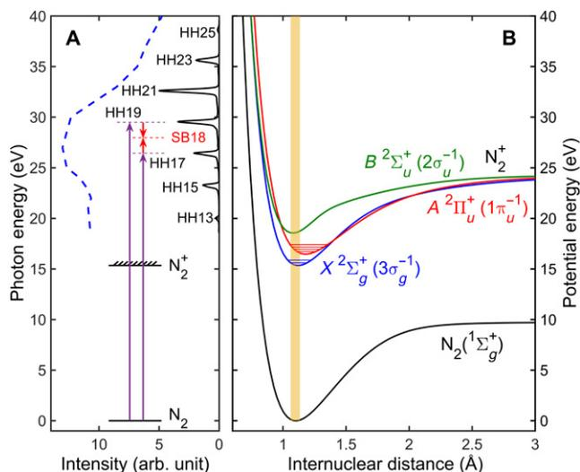
**Figure 5.3:  $N_2$  photoionisation scheme.** A) Harmonics of orders 13-25 are used to probe the  $3\sigma_g$  shape resonance in  $N_2^+$  using the RABBIT technique, indicated in violet (XUV pump) and red (IR probe) arrows. Blue dashed line: photoionisation cross-section. B) Potential energy curves of the ground state of  $N_2$ . Yellow-shaded area: Franck-Condon region. Adapted from Article IV.
