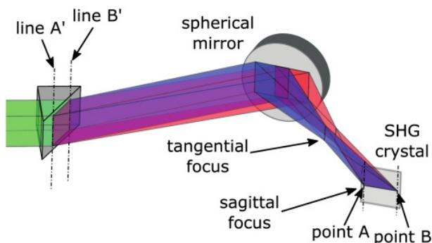
**Figure 3.12: A new design for the single-shot d-scan.** The beam is focused in an off-axis geometry, causing strong astigmatism. Imaging is done in one focal plane, and SHG in the other. Reproduced with permission from Article II.
