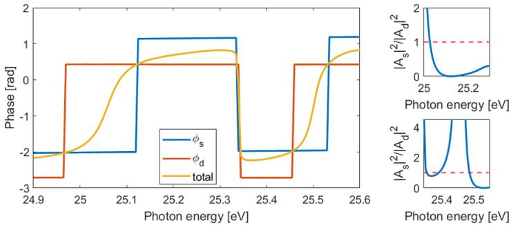
**Figure 5.14: Calculated angle-integrated  $s$  and  $d$  channel phase and relative strength.** The position and slope of the total phase variations are determined by the phases and relative strength of the  $s$  and the  $d$  channel. The red dashed line in the panels on the right indicates equal  $s$  and  $d$  channel amplitudes.
