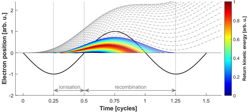
**Figure 2.3:** Classical electron trajectories in HHG. Black: driving electric field (arbitrary units). Colour: long and short recombining trajectories, resulting in photon emission. Gray: trajectories of electrons that do not return to the parent ion. The depicted process repeats every half-cycle of the laser field.
