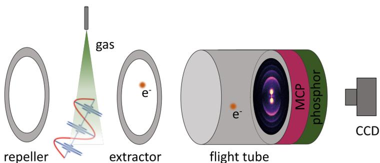
**Figure 4.7:** Principle of VMIS. An electrostatic lens made up of annular electrodes guides electrons towards an MCP followed by a phosphor screen and a camera. Same-energy electrons form ring-like structures on the detector.
