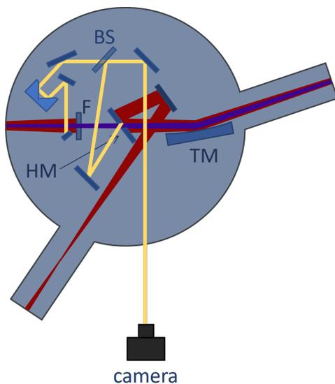
**Figure 4.5: Stabilisation interferometer - part of the beam path not shared with the pump-probe interferometer.** A small portion of the pump beam is taken out before the IR-blocking filter; in the probe arm, a small leakage through the recombination mirror hole is taken. BS recombines the two and the camera records the interference pattern to provide input for the delay stabilisation feedback loop. Note that the angle of HM is exaggerated for easier beam path illustration.
