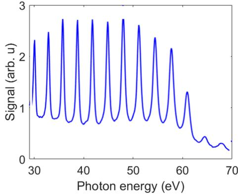
**Figure 2.1: Experimental HHG spectrum.** A plateau region, featuring approximately constant conversion efficiency, is followed by a sharp efficiency-drop called cut-off. The lowest-order harmonics, which exhibit perturbative behaviour, are rarely used in experiments and are thus usually not recorded.
