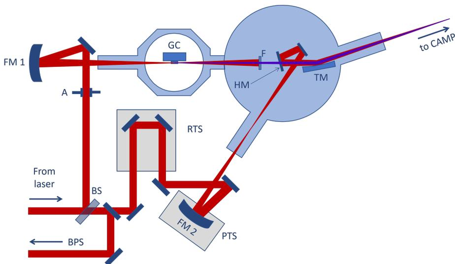
**Figure 4.4: RABBIT interferometer.** BS - beamsplitter, A - aperture, FM - focusing mirror, GC - generation cell, F - filter, HM - holey mirror, TM - toroidal mirror, BPS - beam-pointing stabilisation, RTS - rough translation stage, PTS - precision translation stage, CAMP - Chamber for Atomic and Molecular Physics, where interaction with target gas and photoelectron detection take place.
