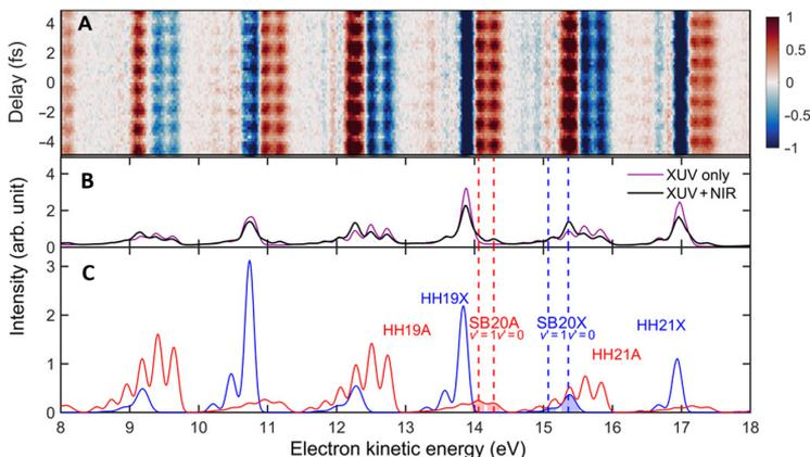
**Figure 5.4: Photoelectron spectra in N<sub>2</sub>.** A) Differential RABBIT spectrogram, obtained as a difference of XUV+NIR and XUV-only spectrograms. B) Photoelectron spectrum (PES) for XUV-only (violet) and XUV+NIR (black) photoionisation, averaged over all relative delays. C) Theoretical PES for XUV+NIR photoionisation to the X (blue) and A (red) states. Adapted from Article IV.
